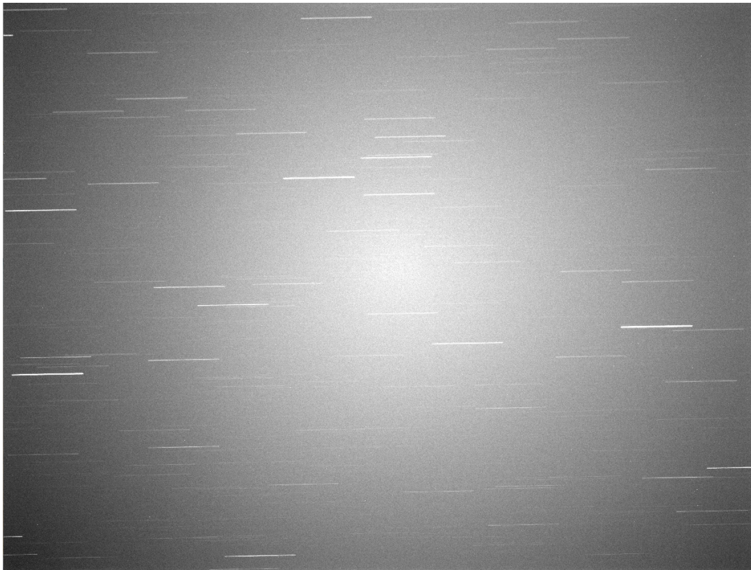
Figure 2.24: An example flat with streaks due to stars being visible when the sky flat was taken. This flat would be rejected because it has too many streaks. The exposure time was 60 seconds, which corresponds to streaks with lengths of about 300 pixels.
