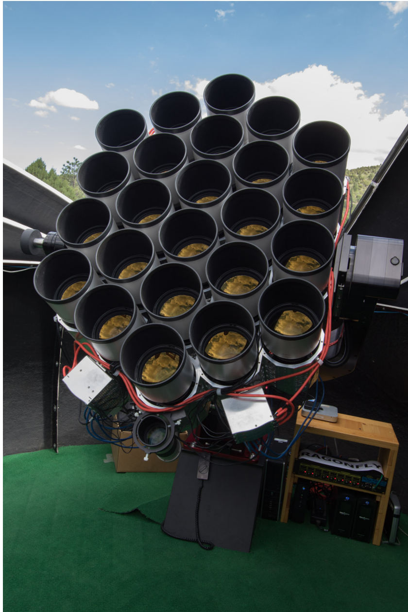
Figure 1.4: Image of one of two 24-lens array mounts of the Dragonfly Telephoto Array.
